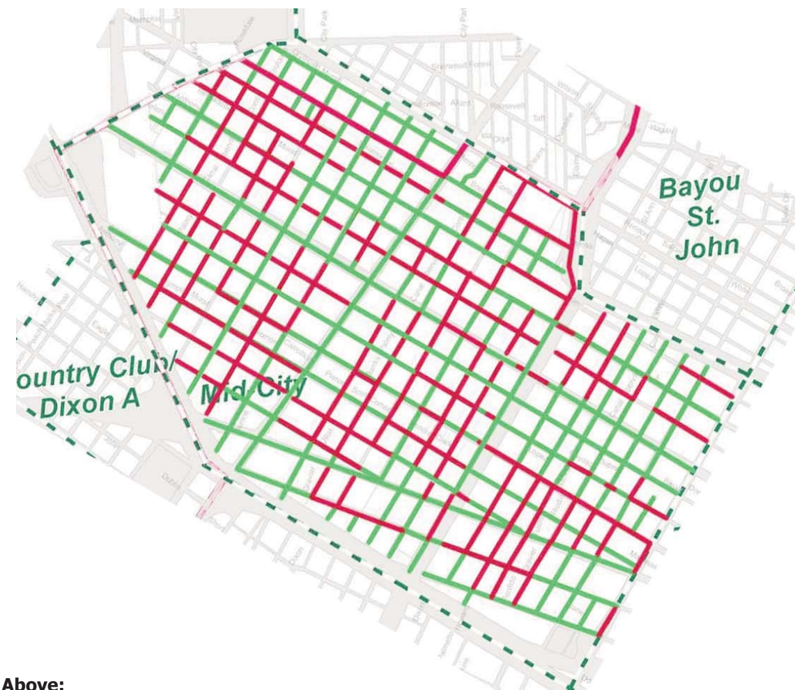
Above: Mid-City Street Survey showing the condition of the streets in the neighborhood. RED - Poor Condition GREEN - Fair/Good Condition
