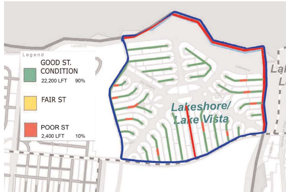
Above: Lake Vista Street Survey showing the condition of the streets in the neighborhood
